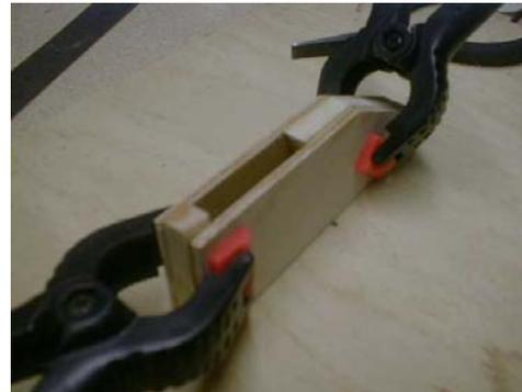
*Finbox Assembly being glued together after having been coated on the inside with epoxy resin and sanded smooth*
