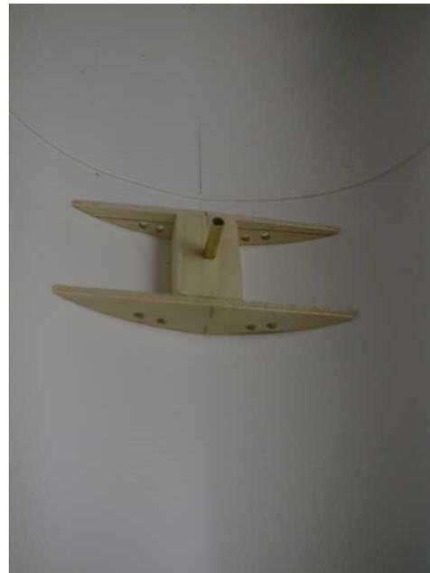
*Lateral Rudder Block support bracing*
