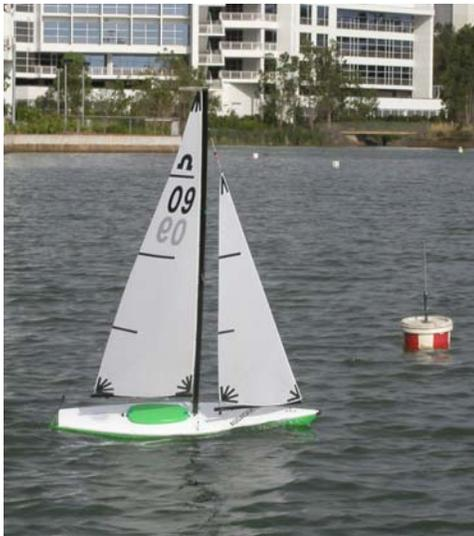
*Note curvature of sails along the foot (bottom of sail) also offset and position of Main Boom, Jib Boom relevant to the centre line of the boat. Allow the main boom to point at the back corner of the boat when hauled hard in.*
