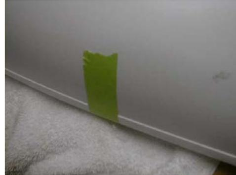
*Taping deck to hull after glueing with polystyrene glue*
