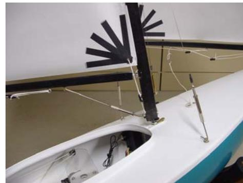
*Simple Gooseneck/Vang Assembly manufactured from a Sails etc..brand large stainless steel sidestay tensioner and bent stainless steel welding wire gooseneck/van pivot epoxied into mast*
