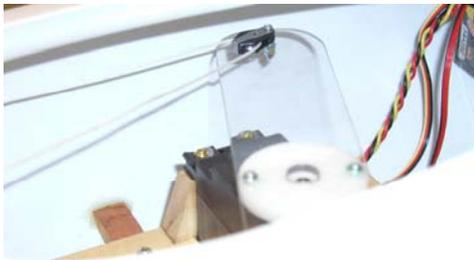
*Lever arm pulley attached to lever arm.*
