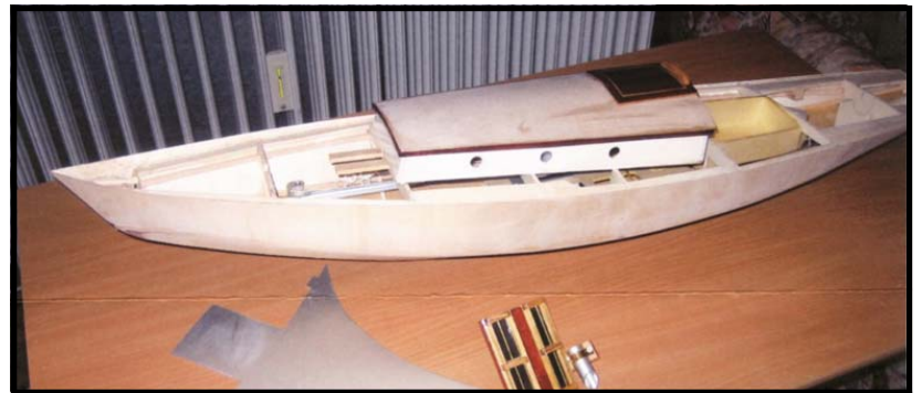
This picture shows off the simple but effective hull and deckhouse construction.
