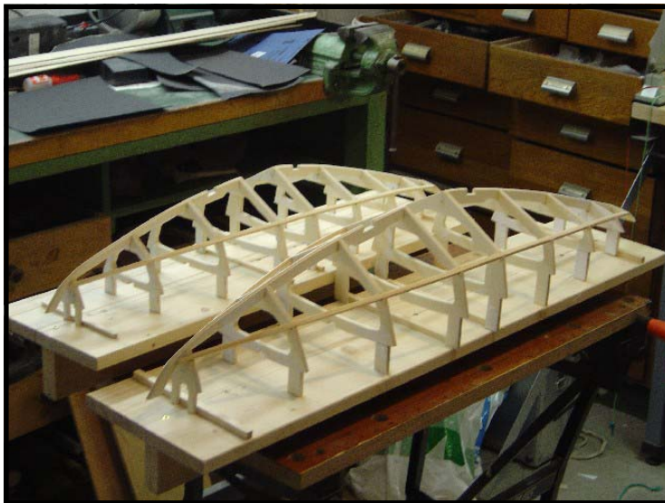
8 Ribs, keel and chines in position.
