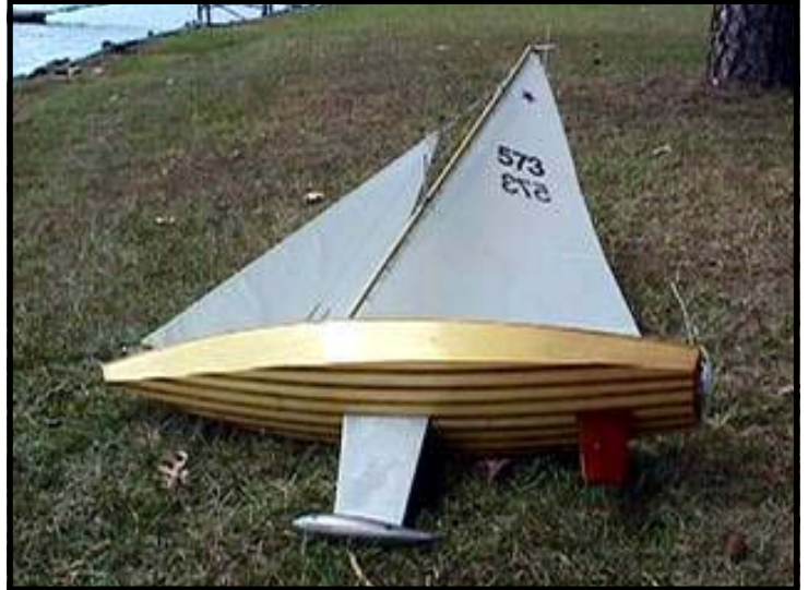
One concession to the Star 45's scale appearance is the fin, bulb and rudder.
