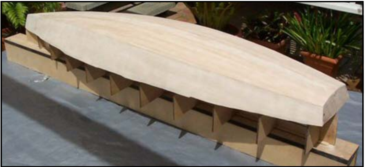
Completed Star 45 Balsa wood hull ready for glassing.
