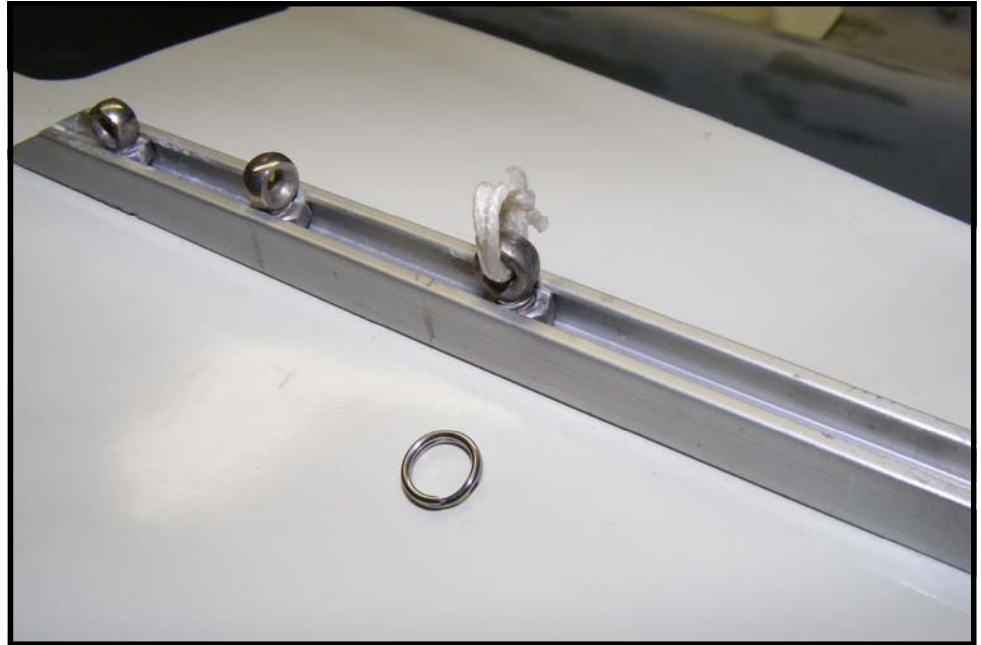
Sample of the culprit concerned in the article along with the temporary (now permanent) dyneema cord repair.
