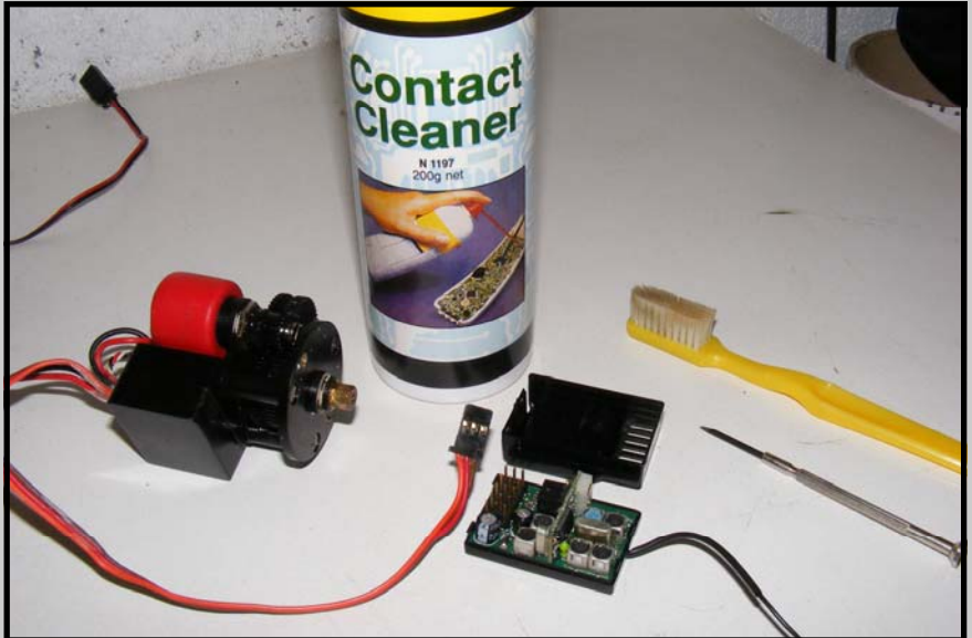
Contact Cleaner used to clean up the corroded contacts on the wind and receiver.
